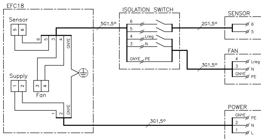
Connect the EFC18 and the temperature sensor as in the diagram below (RSHT).
